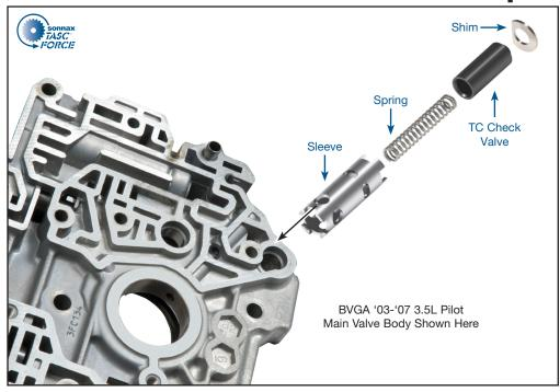
An overheating torque converter is a common problem in Honda vehicles equipped with a four- or five-speed automatic transmission. This condition can be caused by a worn or stuck TC check valve, which reduces the pressure in the torque converter and leads to excess heat buildup.
