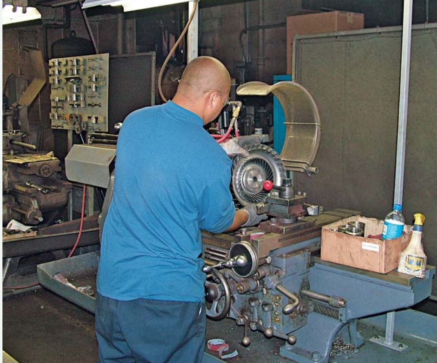
Before going to the rebuild area, converters are opened and machined to specification.
