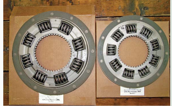
Building on the company's expertise with bonding friction material, a new CVC product line is relined clutch dampers for Allison transmissions.
